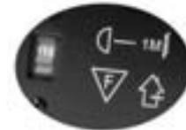
Not all fixtures have a voltage select switch. Please be sure to connect to the proper voltage.
